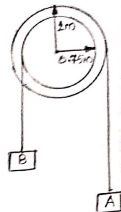
⑨ A pulley 2m in diameter is connected to a shaft which makes 240 rpm. Find the linear velocity of a particle on the periphery of the pulley.
