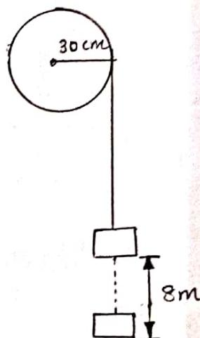
a) ∴ angular acceleration of pulley;  $\alpha = \underline{\underline{3.33 \text{ rad/s}^2}}$
